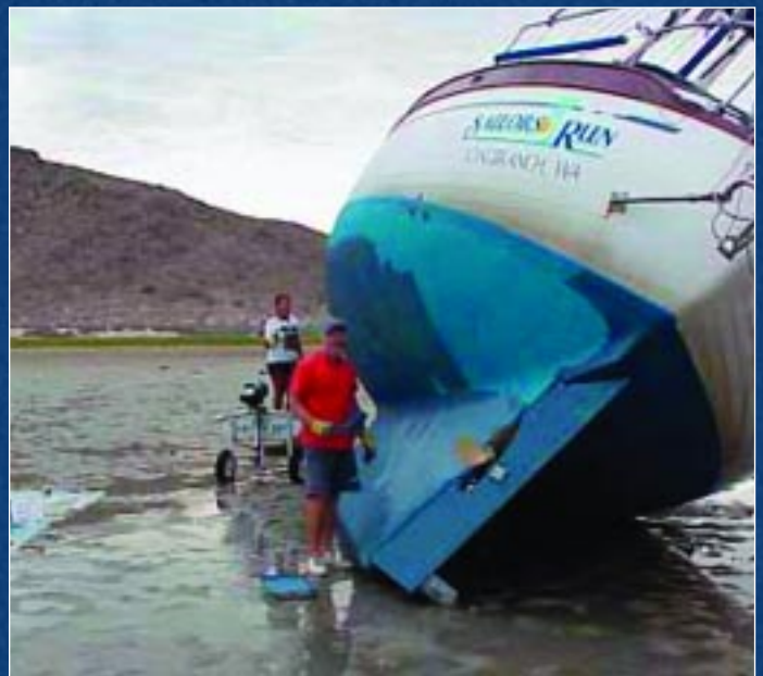
Careening a sailboat Caution: Don't try this yourself! Go to a boat repair yard, instead.
