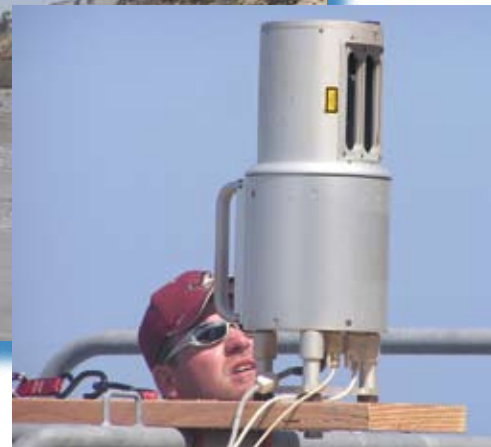
LIDAR scanning of a section of Solana Beach bluffs. Photos CSG archives
