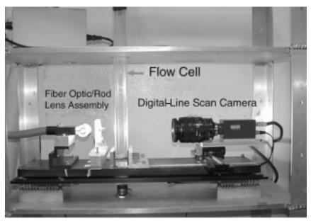
REFLICS: Water from CUFES concentrator passes upward through the flow cell at 20 l min<sup>-1</sup> and on to CUFES sample collector (see illustration on previous page). Particles are backlit by the illuminator and imaged by the line-scan camera. Data are transferred from camera to computer for real-time acquisition and analysis. Photo: Jesse Powell, UC San Diego
