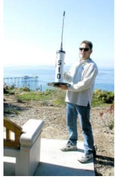
Drifters, such as the one displayed above, are made of PVC piping and are about 1.2 meters tall.
