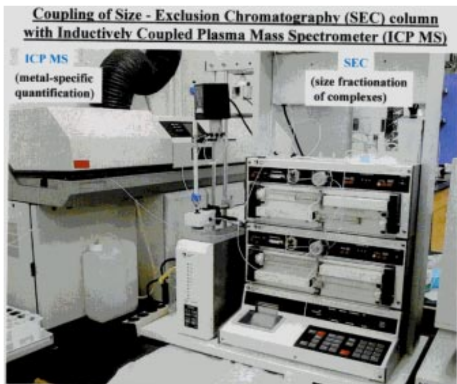
It takes very complex instrumentation to measure the different metal-containing compounds in water. Here is an instrument used by Dr. Janet Hering of the California Institute of Technology to measure copper and nickel in laboratory water samples. Photo: California Institute of Technology.
