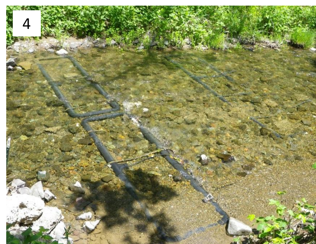
Figure 4. A fraction of all juvenile hatchery coho released into Mill Creek each year are PIT-tagged. When a tagged coho pass by an antenna's transceiver field, a reader records tag number, date and time.
