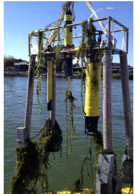
Recovery of flow and sediment mooring after the first field experiment (09/2016) on the Sacramento River at Rio Vista. Ivy Huang
