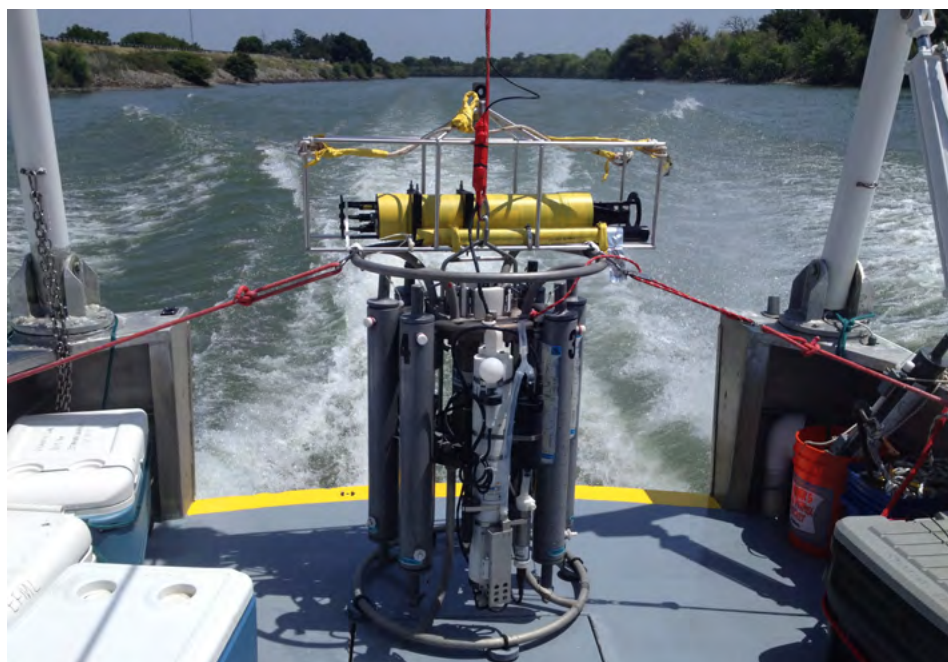
Researchers collected high-resolution fluid and sediment data at three sites around the Delta. They used advanced particle sizing instruments shown above to measure changes in flocculation properties such as such as floc size, density and fall velocity. Ivy Huang
