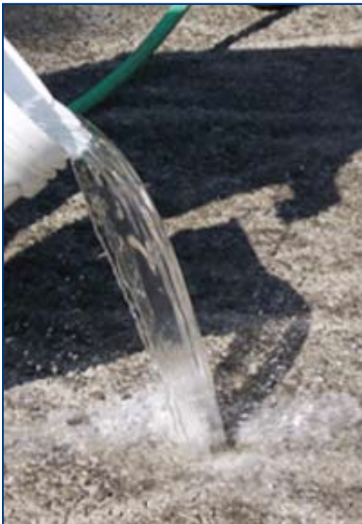
Water poured onto pervious concrete filters through to recharge groundwater.
