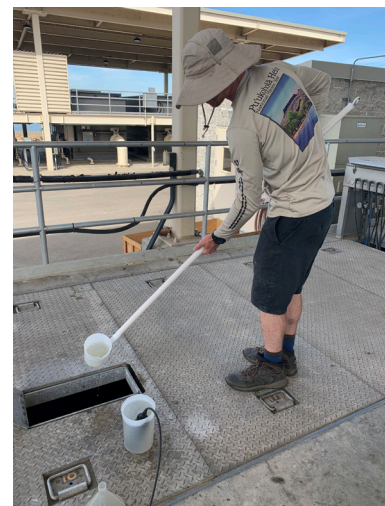
LEFT: Delta Science Fellow Joseph Fackrell sets up equipment to sample the San Joaquin river from the Sherman Island levee. ABOVE: Joseph samples treated wastewater at White Slough Wastewater Pollution Control Facility with a dipping cup. Christina Richardson
