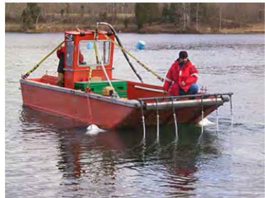
Figure 4-1. Watercraft equipped with diffuser system in Millbrook Quarry. Photo Credit: Virginia Department of Game and Inland Fisheries
