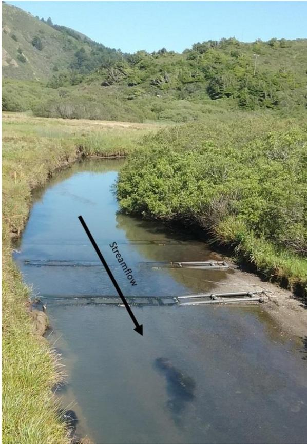
**Figure 2. Paired flat-plate antenna array on Willow Creek.**
