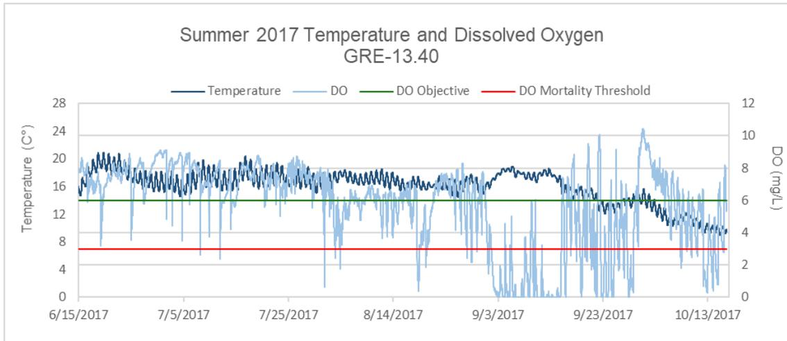
FIGURE 11. CONTINUOUS TEMPERATURE AND DISSOLVED OXYGEN MEASUREMENTS FROM GAGE POOL IN THE GRE-13.40 STUDY REACH, PLOTTED WITH REGIONAL DO OBJECTIVE (6.0 MG/L) AND SALMONID MORTALITY THRESHOLD (3.0 MG/L), SUMMER 2017.
