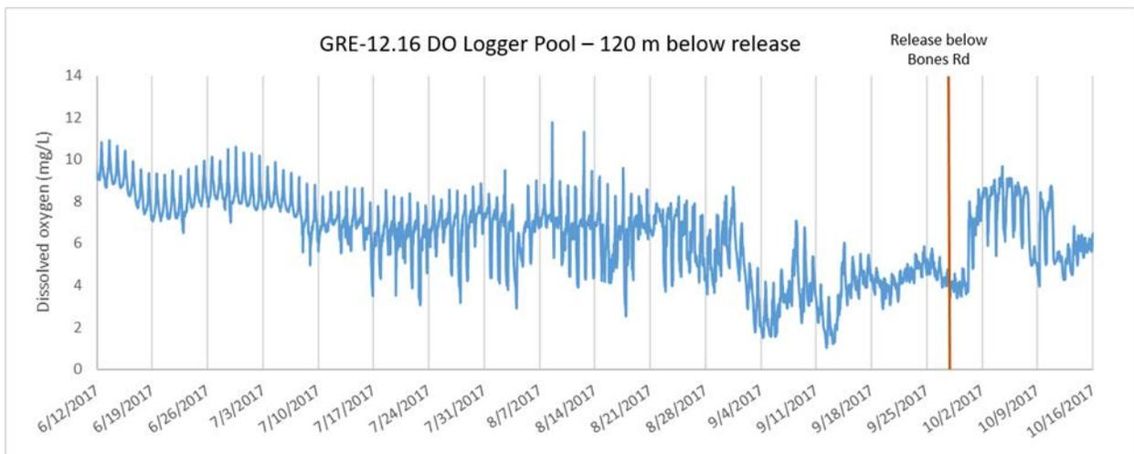
FIGURE 46. DO MEASUREMENTS FROM CONTINUOUS LOGGER IN STUDY POOL 120 METERS DOWNSTREAM OF THE FLOW RELEASE INITIATED ON UPPER GREEN VALLEY CREEK ON SEPTEMBER 28, 2017. RED LINE INDICATES RELEASE DATE. NOTE INCREASE IN DO AFTER FLOW AUGMENTATION.
