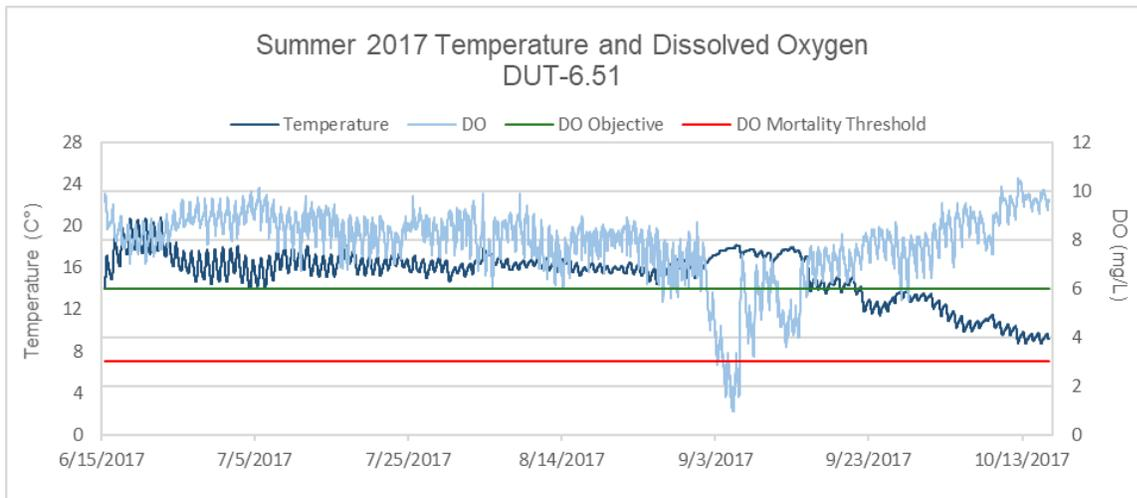
**FIGURE 9. CONTINUOUS TEMPERATURE AND DISSOLVED OXYGEN MEASUREMENTS FROM GAGE POOL IN THE DUT-6.51 STUDY REACH, PLOTTED WITH REGIONAL DO OBJECTIVE (6.0 MG/L) AND SALMONID MORTALITY THRESHOLD (3.0 MG/L), SUMMER 2017.**
