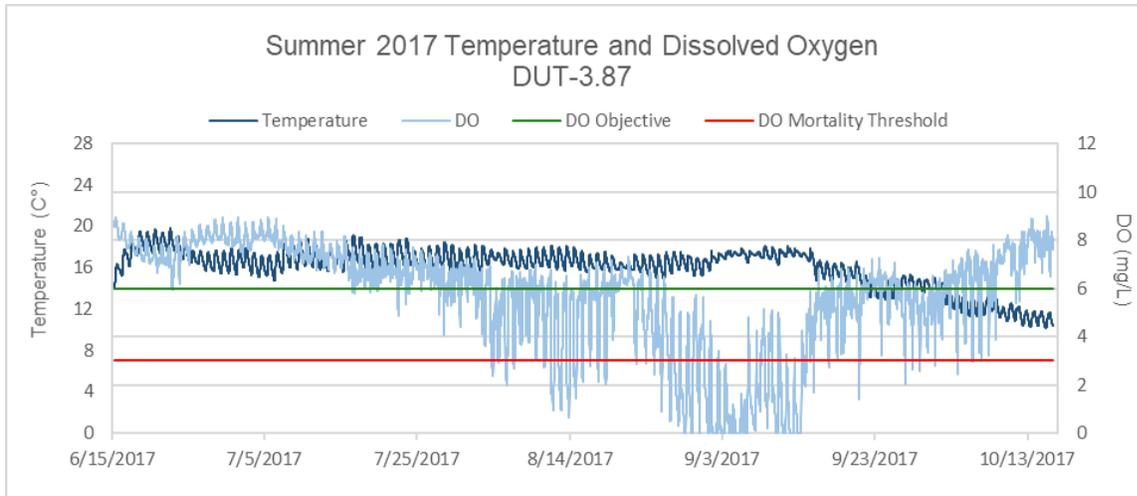
**FIGURE 8. CONTINUOUS TEMPERATURE AND DISSOLVED OXYGEN MEASUREMENTS FROM GAGE POOL IN THE DUT-3.87 STUDY REACH, PLOTTED WITH REGIONAL DO OBJECTIVE (6.0 MG/L) AND SALMONID MORTALITY THRESHOLD (3.0 MG/L), SUMMER 2017.**
