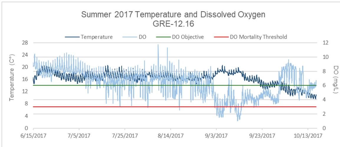
**FIGURE 10. CONTINUOUS TEMPERATURE AND DISSOLVED OXYGEN MEASUREMENTS FROM GAGE POOL IN THE GRE-12.16 STUDY REACH, PLOTTED WITH REGIONAL DO OBJECTIVE (6.0 MG/L) AND SALMONID MORTALITY THRESHOLD (3.0 MG/L), SUMMER 2017.**
