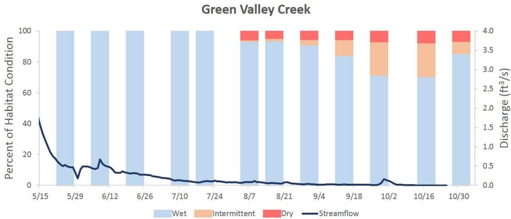
**FIGURE 38. STREAMFLOW AND PERCENT OF WET, INTERMITTENT AND DRY STREAM HABITAT OBSERVED ON BIWEEKLY SURVEYS ON GREEN VALLEY CREEK, 2017. STREAMFLOW DATA WAS GENERATED FROM GAGE IN REACH GRE-13.40.**
