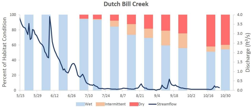
**FIGURE 37. STREAMFLOW AND PERCENT OF WET, INTERMITTENT AND DRY STREAM HABITAT OBSERVED ON BIWEEKLY SURVEYS ON DUTCH BILL CREEK, 2017. STREAMFLOW DATA WAS GENERATED FROM GAGE IN REACH DUT-3.87.**
