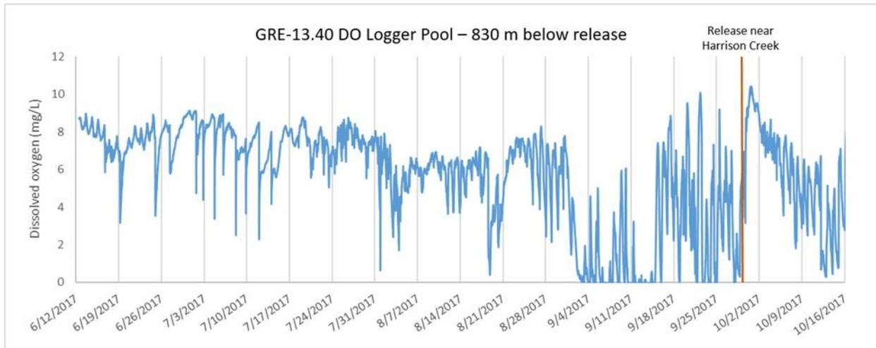
**FIGURE 47. DO MEASUREMENTS FROM CONTINUOUS LOGGER IN STUDY POOL 830 METERS DOWNSTREAM OF THE FLOW RELEASE INITIATED ON UPPER GREEN VALLEY CREEK ON SEPTEMBER 29, 2017. RED LINE INDICATES RELEASE DATE. NOTE INCREASE IN DO AFTER FLOW AUGMENTATION.**
