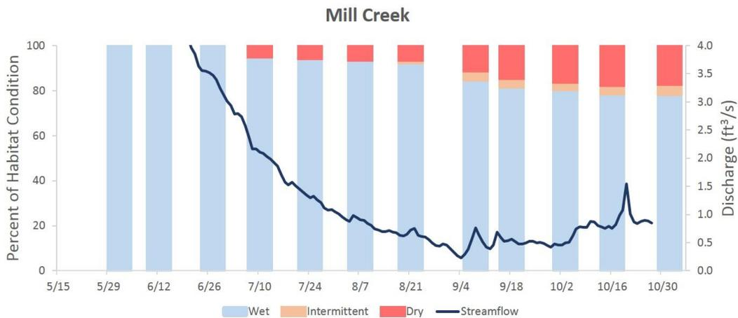
**FIGURE 39. STREAMFLOW AND PERCENT OF WET, INTERMITTENT AND DRY STREAM HABITAT OBSERVED ON BIWEEKLY SURVEYS ON MILL CREEK, 2017. STREAMFLOW DATA WAS GENERATED FROM GAGE IN REACH MIL-6.10.**
