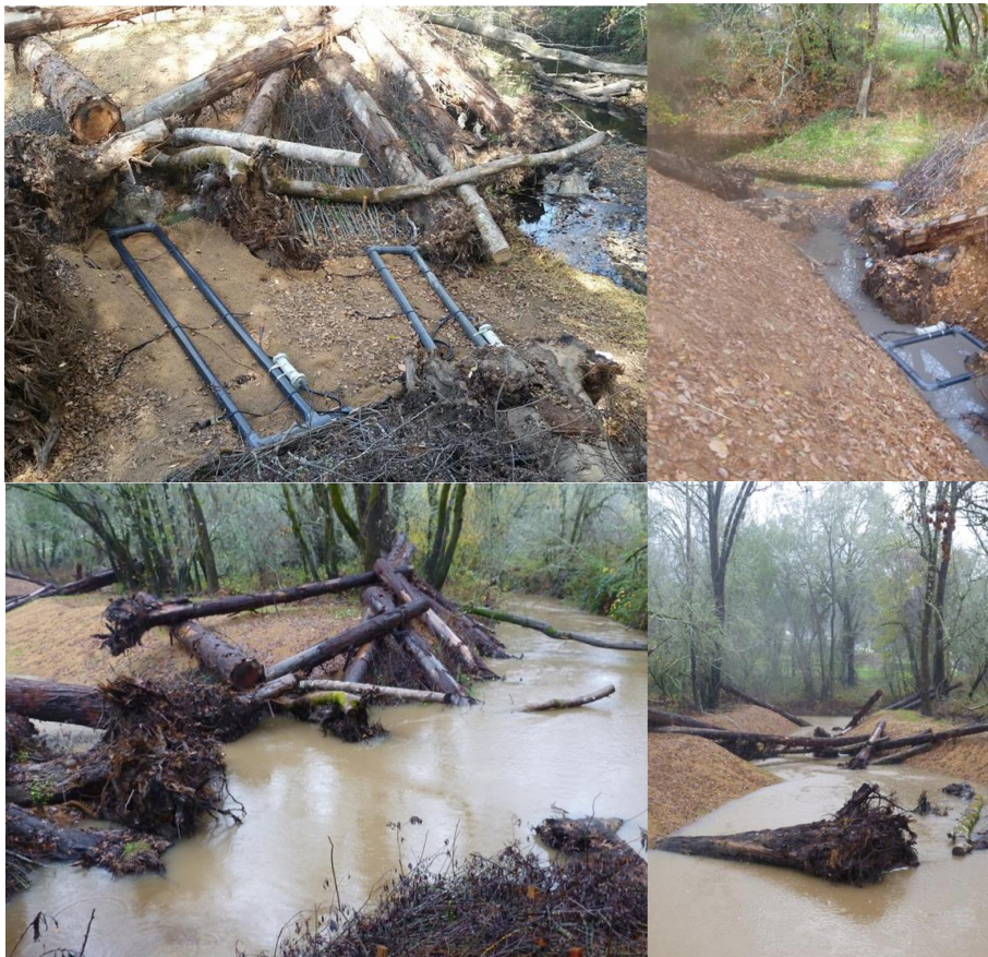
Figure 3. Off-Channel PIT antenna sites prior to winter flows (top two photos) and after the habitat was activated (bottom two photos). The off-channel inlet array, GRE-6.09, is on the right and the off-channel outlet array, GRE-6.03, is on the left.
