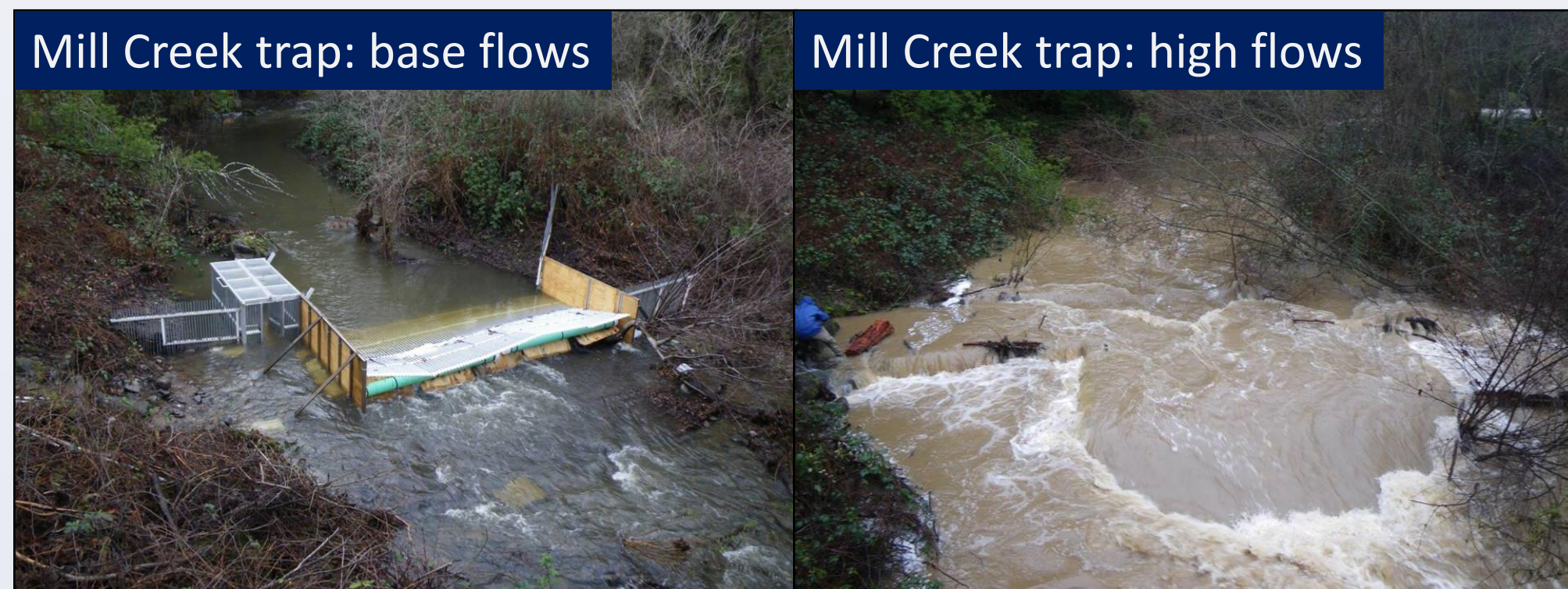
Figure 1. Adult trap on Mill Creek during base flow and storm flow conditions.
