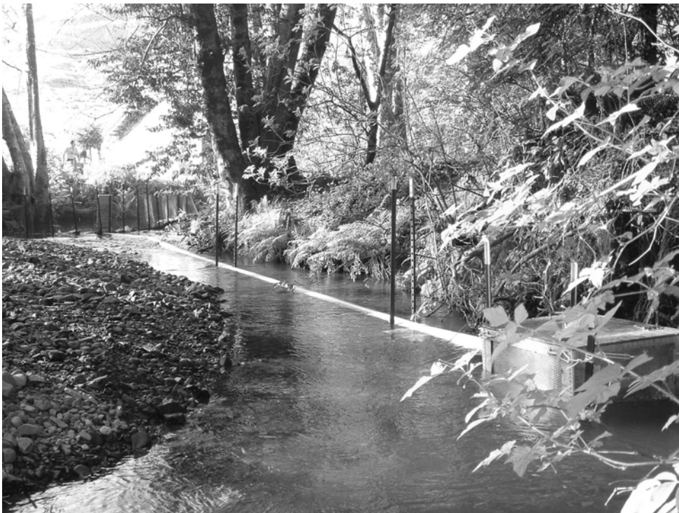
Figure 5. Trap designs used on Mill Creek (a) and Sheephouse Creek (a) in 2005. The funnel trap used on Mill was similar to designs used on Ward and Green Valley while the pipe trap design was only used on Sheephouse.
