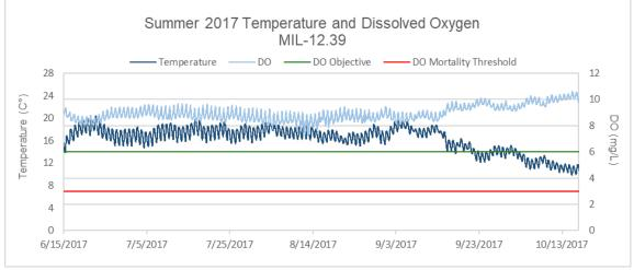
FIGURE 13. CONTINUOUS WATER TEMPERATURE AND DISSOLVED OXYGEN MEASUREMENTS FROM GAGE POOL IN THE MIL-12.39 STUDY REACH, PLOTTED WITH REGIONAL DO OBJECTIVE (6.0 MG/L) AND SALMONID MORTALITY THRESHOLD (3.0 MG/L), SUMMER 2017.
