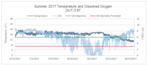
FIGURE 8. CONTINUOUS TEMPERATURE AND DISSOLVED OXYGEN MEASUREMENTS FROM GAGE POOL IN THE DUT-3.87 STUDY REACH, PLOTTED WITH REGIONAL DO OBJECTIVE (6.0 MG/L) AND SALMONID MORTALITY THRESHOLD (3.0 MG/L), SUMMER 2017.
