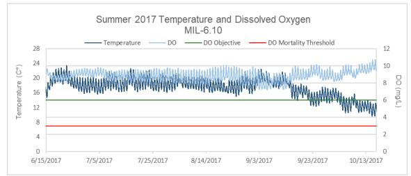
FIGURE 12. CONTINUOUS TEMPERATURE AND DISSOLVED OXYGEN MEASUREMENTS FROM GAGE POOL IN THE MIL-6.10 STUDY REACH, PLOTTED WITH REGIONAL DO OBJECTIVE (6.0 MG/L) AND SALMONID MORTALITY THRESHOLD (3.0 MG/L), SUMMER 2017.
