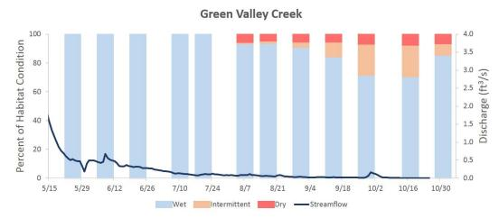
FIGURE 38. STREAMFLOW AND PERCENT OF WET, INTERMITTENT AND DRY STREAM HABITAT OBSERVED ON BIWEEKLY SURVEYS ON GREEN VALLEY CREEK, 2017. STREAMFLOW DATA WAS GENERATED FROM GAGE IN REACH GRE-13.40.
