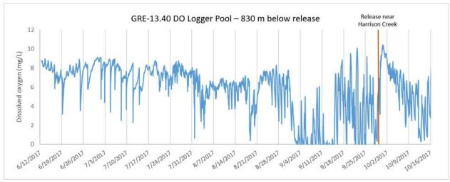
FIGURE 47. DO MEASUREMENTS FROM CONTINUOUS LOGGER IN STUDY POOL 830 METERS DOWNSTREAM OF THE FLOW RELEASE INITIATED ON UPPER GREEN VALLEY CREEK ON SEPTEMBER 29, 2017. RED LINE INDICATES RELEASE DATE. NOTE INCREASE ID DO AFTER FLOW AUGMENTATION.
