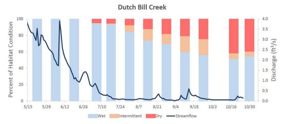
FIGURE 37. STREAMFLOW AND PERCENT OF WET, INTERMITTENT AND DRY STREAM HABITAT OBSERVED ON BIWEEKLY SURVEYS ON DUTCH BILL CREEK, 2017. STREAMFLOW DATA WAS GENERATED FROM GAGE IN REACH DUT-3.87.
