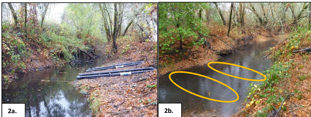
Figure 2a-b. PIT antenna arrays in the main channel of Green Valley Creek. 2a: Array 1, four antenna array. 2b: Array 4, two antenna array with antennas circled in orange.
