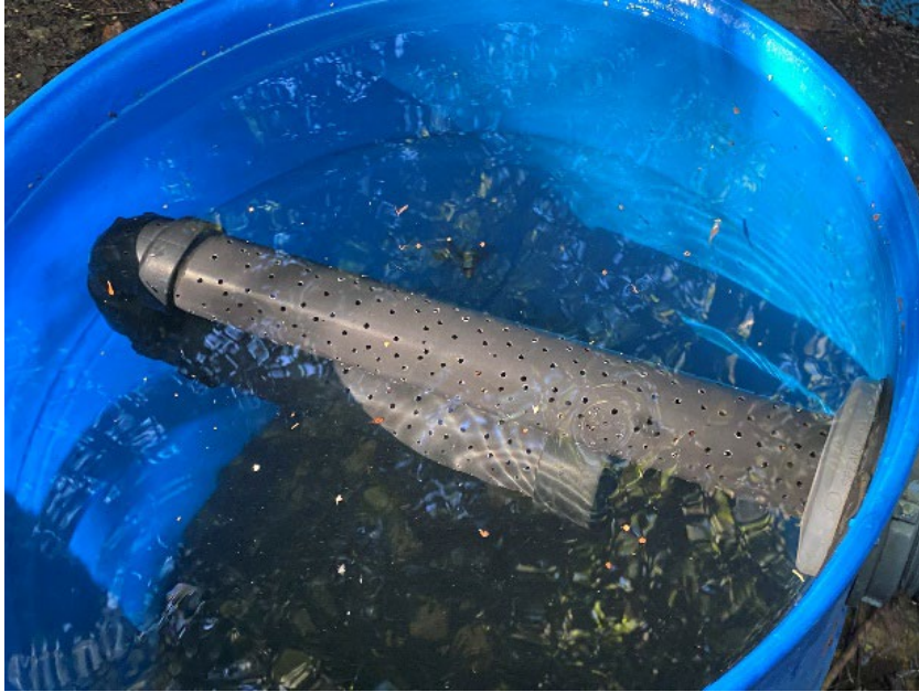
Figure 2. The RSI unit was modified with the installation of a filter on the outflow pipe of the incubation tank around day 10 to prevent the movement of alevin from the incubation tank to the live cart tank.
