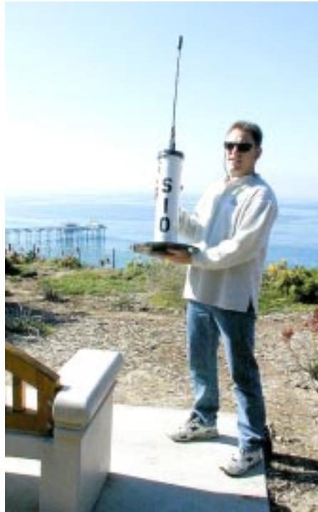
Drifters, such as the one displayed above, are made of PVC piping and are about 1.2 meters tall.
