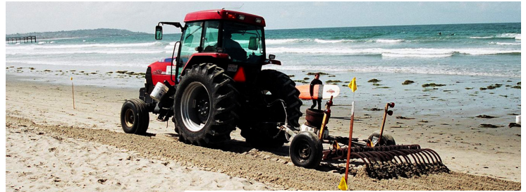
A tractor outfitted with a large metal rake removes wrack from the beach. Karen Martin
