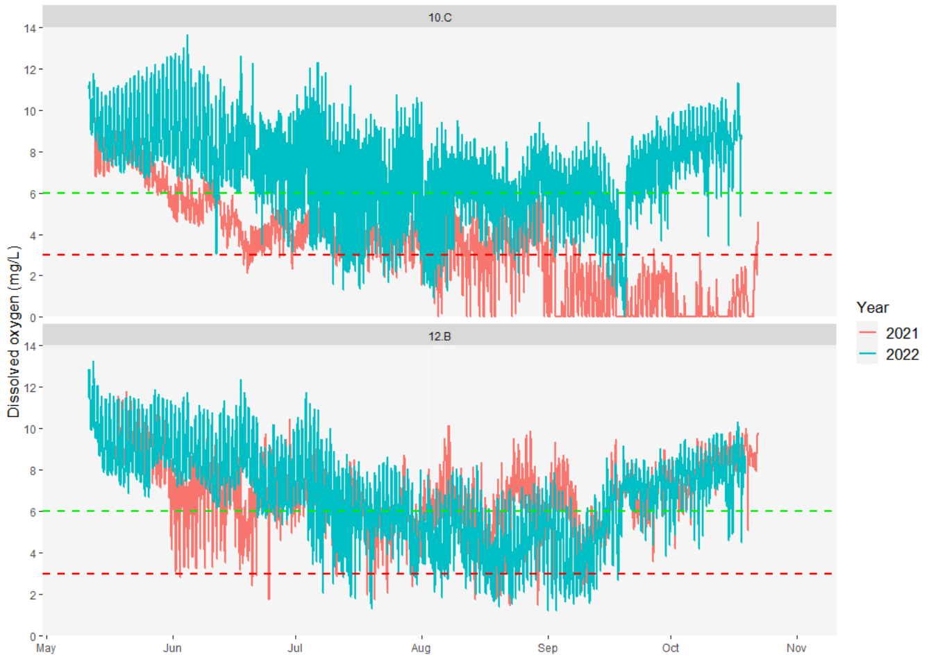
Figure 37. Mark West Creek continuous dissolved oxygen at sites 10.C (top panel) and 12.B (bottom panel), summers 2021 and 2022. Dashed green line represents the regional daily minimum objective of 6.0 mg/L and the dashed red line represents the mortality threshold of 3.0 mg/L.
