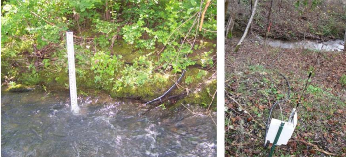
Figure 4 A-B. Streamflow gauges in Grape Creek: (A) Submerged sensor at end of Azonde pressure transducer and staff plate; (B) Azonde antenna and cable
