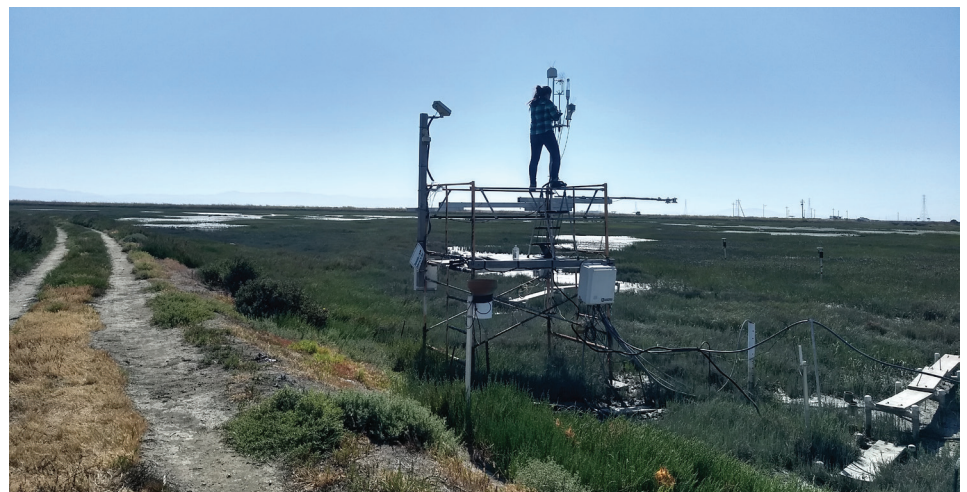
And eddy covariance tower was built in the marsh to collect the data.
