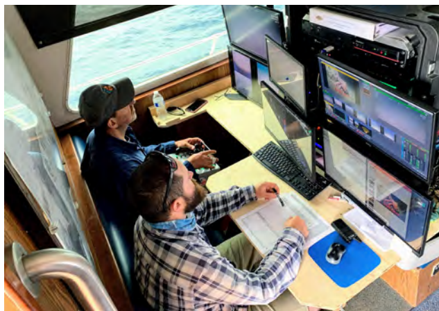
Dirk Rosen (pilot) and Sam Parker (navigation) working together to fly the ROV Beagle along a transect, observing mid-depth rocky reef ecosystems.
