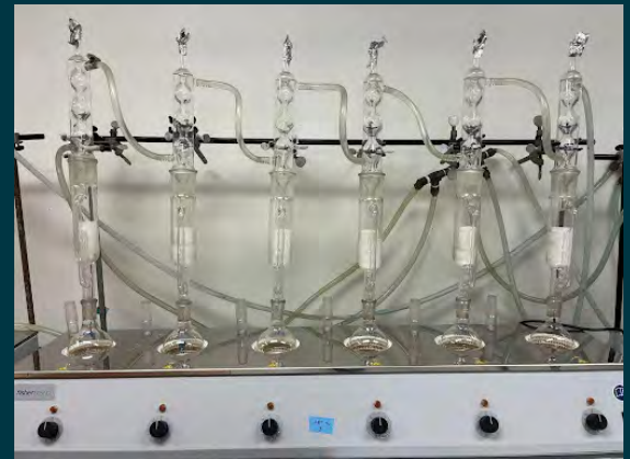
Soxhlet extraction is the first step for extraction of organic contaminants from fish tissues. Specific solvents are used that allow contaminants to move from the tissues to the extract, which will be further purified before analysis.
