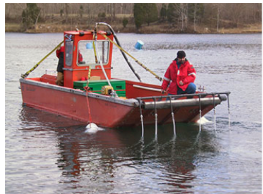
Figure 4-1. Watercraft equipped with diffuser system in Millbrook Quarry. Photo Credit: Virginia Department of Game and Fisheries
