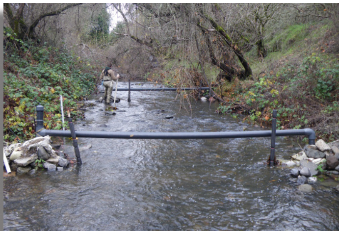
Two PIT tag antennas on Mill Creek are set up in series to estimate capture efficiency and determine which direction the fish is travelling.
