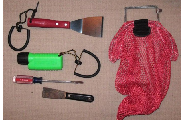
Figure 2-3. Examples of hand-held tools, some brightly colored and with leashes, useful for removing mussels from hard-to-reach places. Dive collection mesh bag useful for holding tools and for collecting removed animals. Photo Credit: Carolynn Culver
