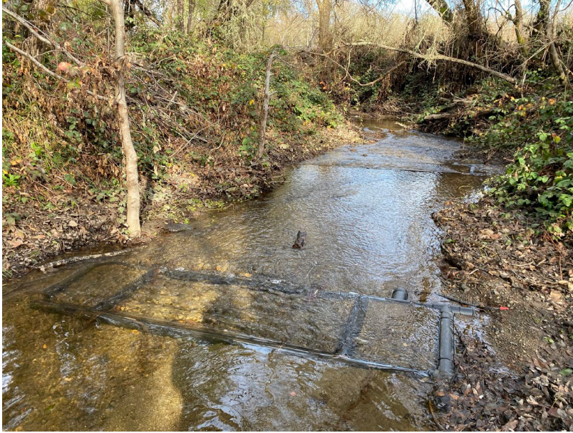
Figure 2. Paired flat-plate antenna array on a Russian River tributary.
