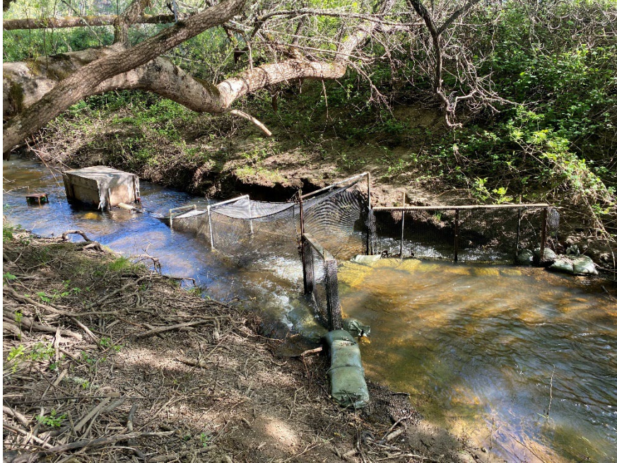
Figure 3. Downstream migrant funnel trap at a new trap site on Green Valley Creek.
