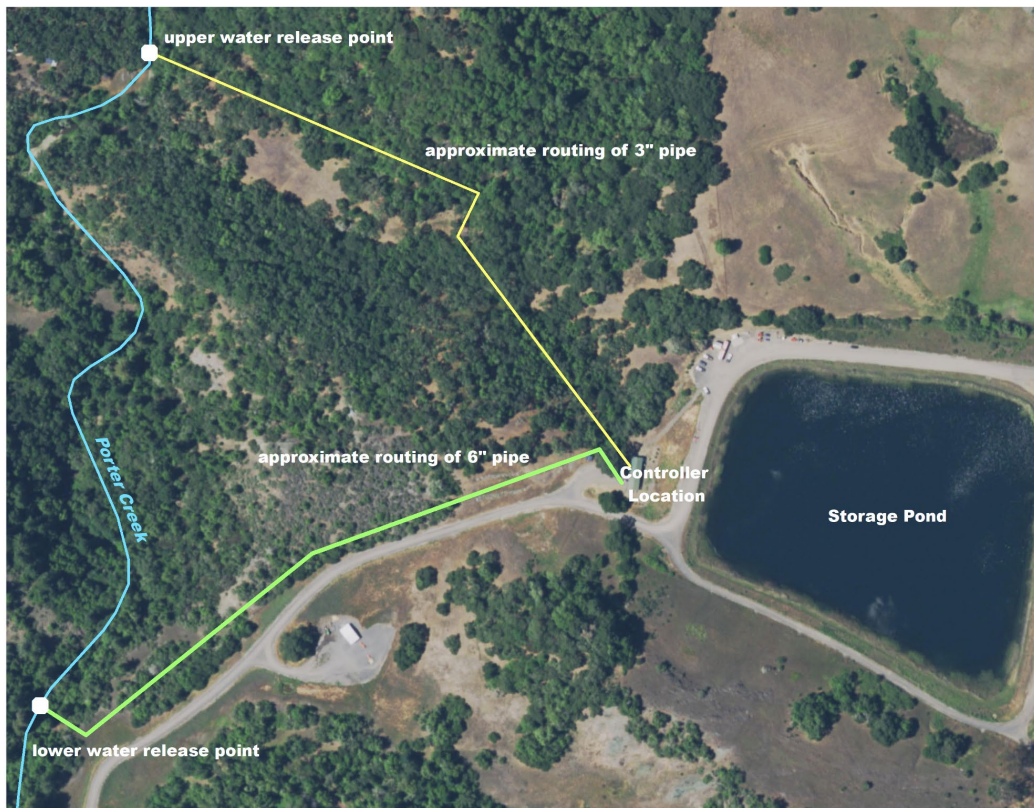
Figure 7. Schematic of approximate locations of pipe and water release points to Porter Creek from the storage pond.
