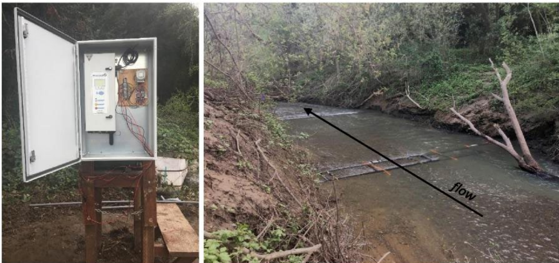
Figure 9. PIT transceiver (left) and antenna array (right) located near the mouth of Porter Creek.
