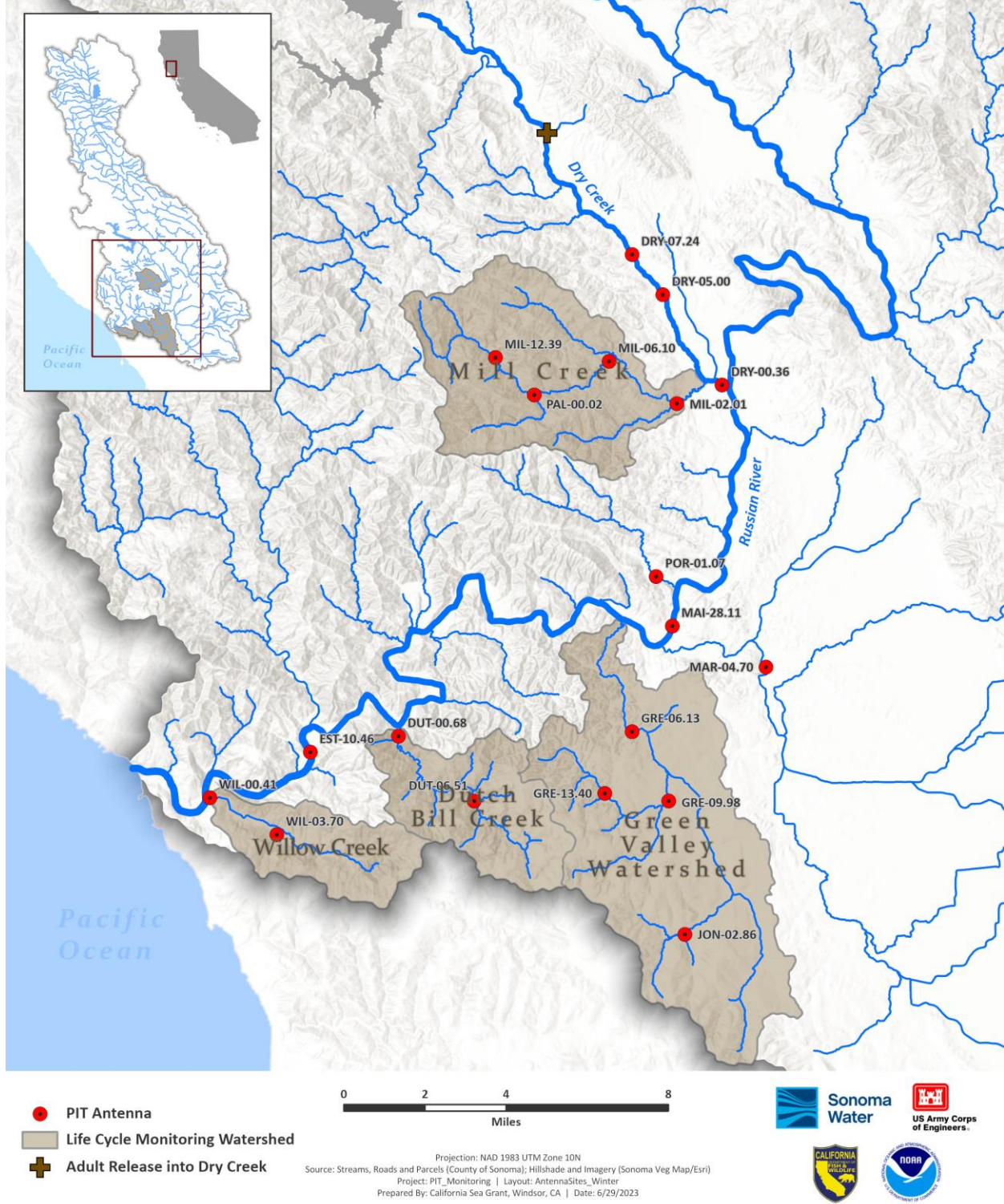
Figure 1. Passive integrated transponder (PIT) antenna and adult release location in the Russian River watershed, winter 2022/23. Labels on antennas include a stream code (first three letters of the stream) and the distance in km from the mouth of that stream.
