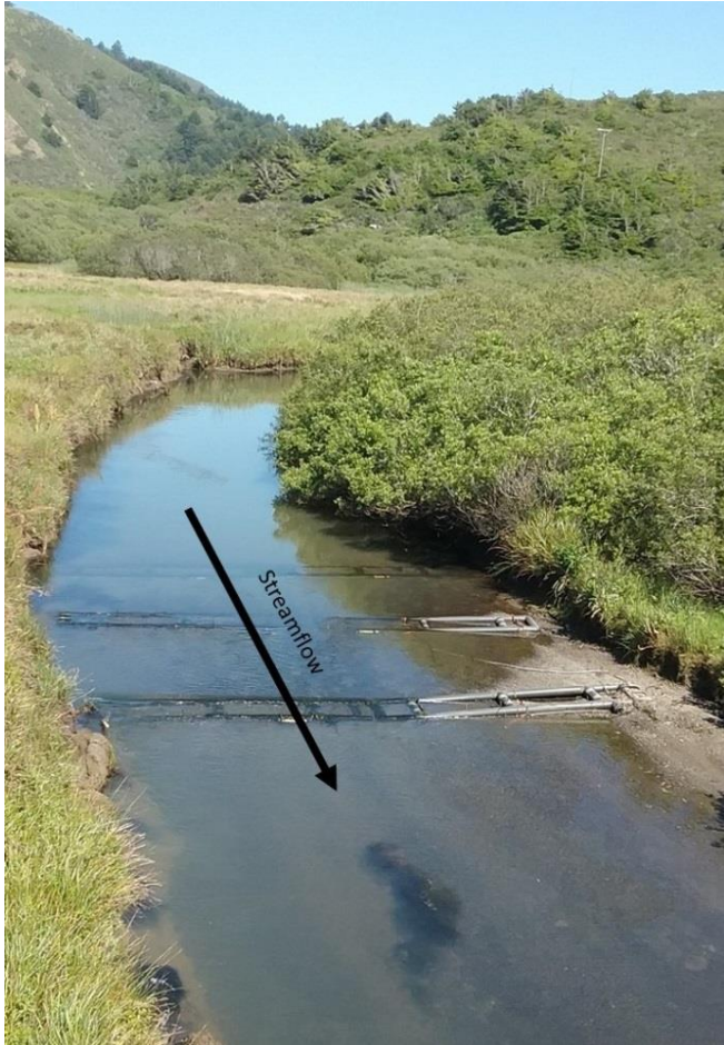
Figure 2. Paired flat-plate antenna array on Willow Creek.
