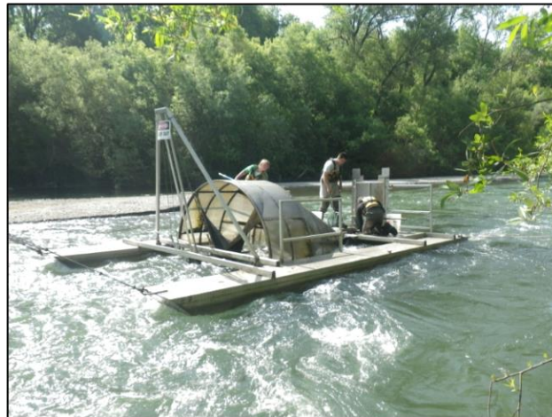
Figure 5. Chinook LCS at Mirabel on the mainstem Russian River: adult underwater video and DIDSON monitoring at fish ladders associated with the Mirabel dam (upper panels) and downstream migrant trap.
