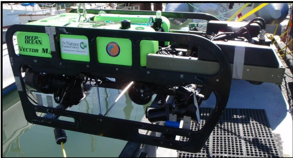
**Figure 2:** The Vector M4 ROV “Beagle” configured for this project with a forward mount to support a down-looking still and video camera and paired lasers in addition to the existing oblique video camera and lasers.
